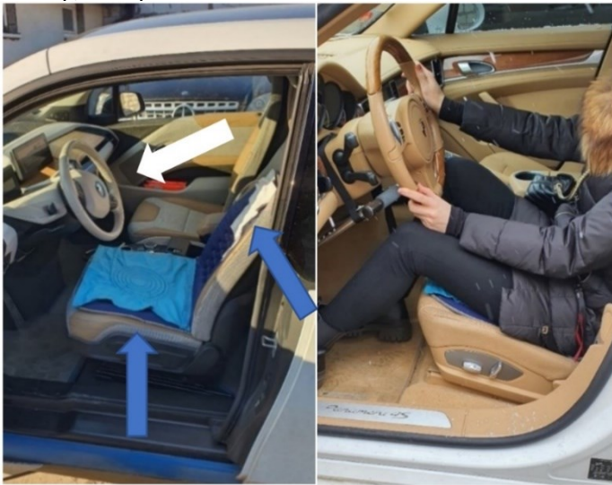
Fig. 4. Sensors integrated in driver seat (blue arrows) and reference sensor (white arrow) to monitor vibrations of combust engines.
